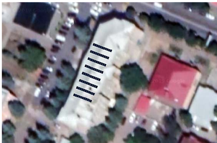
Location of PV modules on the roof of the building
